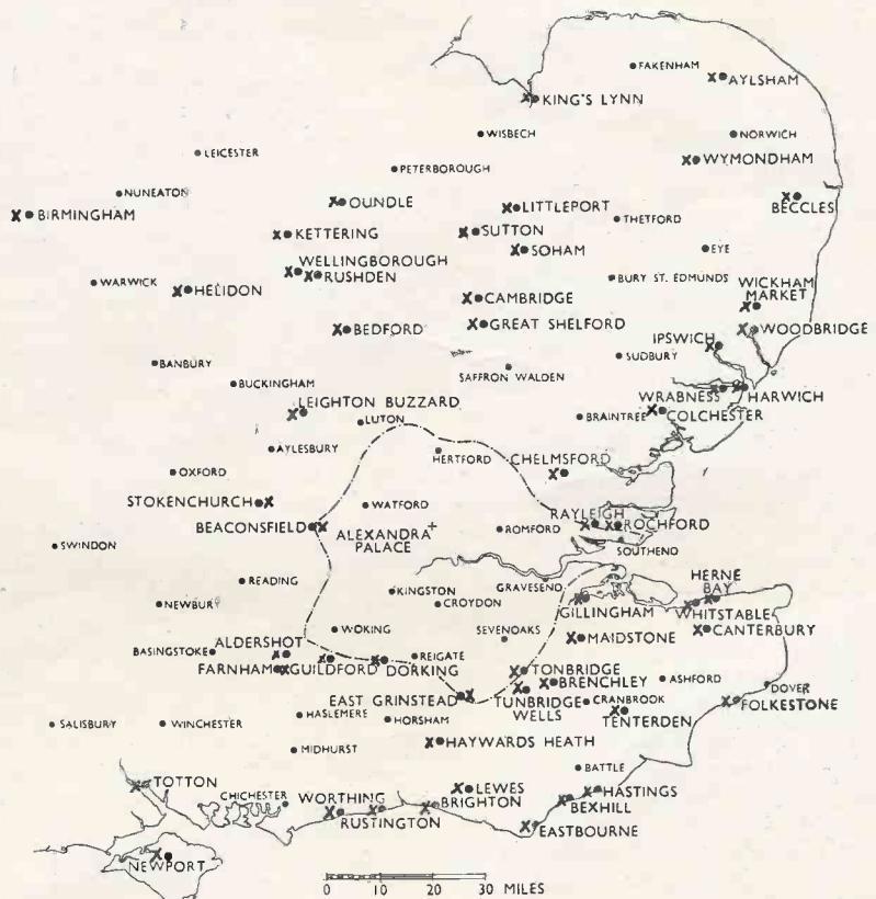
Map of Service Area of London Television Station. - - - - - Outer limit of normal reliable service area. X Localities outside service area where good television reception has been experienced.
