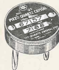
The new Q.C.C. crystal holder fits American type valve holders.
